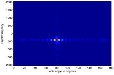
Fig 2: STAP implementation for Doppler frequency vs Look angle plot
